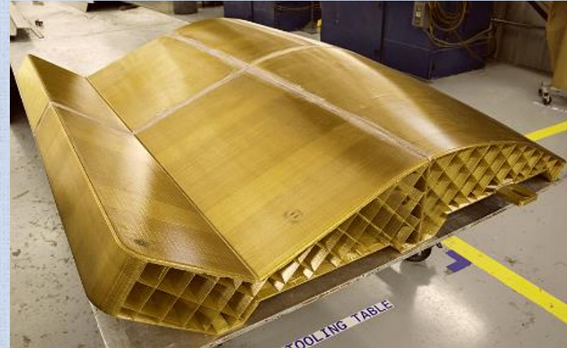
A 3D printed composite layup tool used in the aerospace industry
